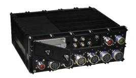
Powered by the 13th Gen Intel® Core™ i7-13800HRE processor (6 performance cores + 8 efficiency cores, 20 threads), Falcon 3R not only builds on the legacy of the Falcon line but takes a decisive leap forward with significantly expanded mezzanine card support—5 x MiniPCle and 2 x XMC slots—making it the most I/O-intensive system in the Falcon family. This advancement allows engineers to deploy a far wider range of I/O modules, ideal for complex mission-critical and data-heavy applications.
